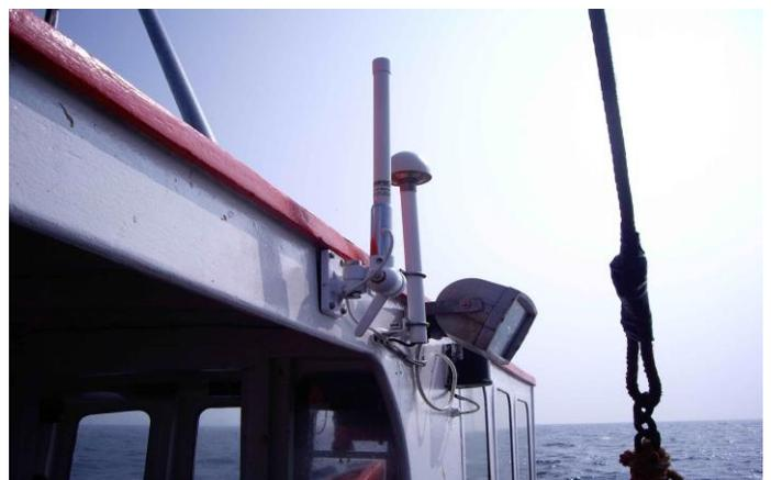
Figure 1: A vessel monitoring device fitted to a fishing vessel (Seafish).
